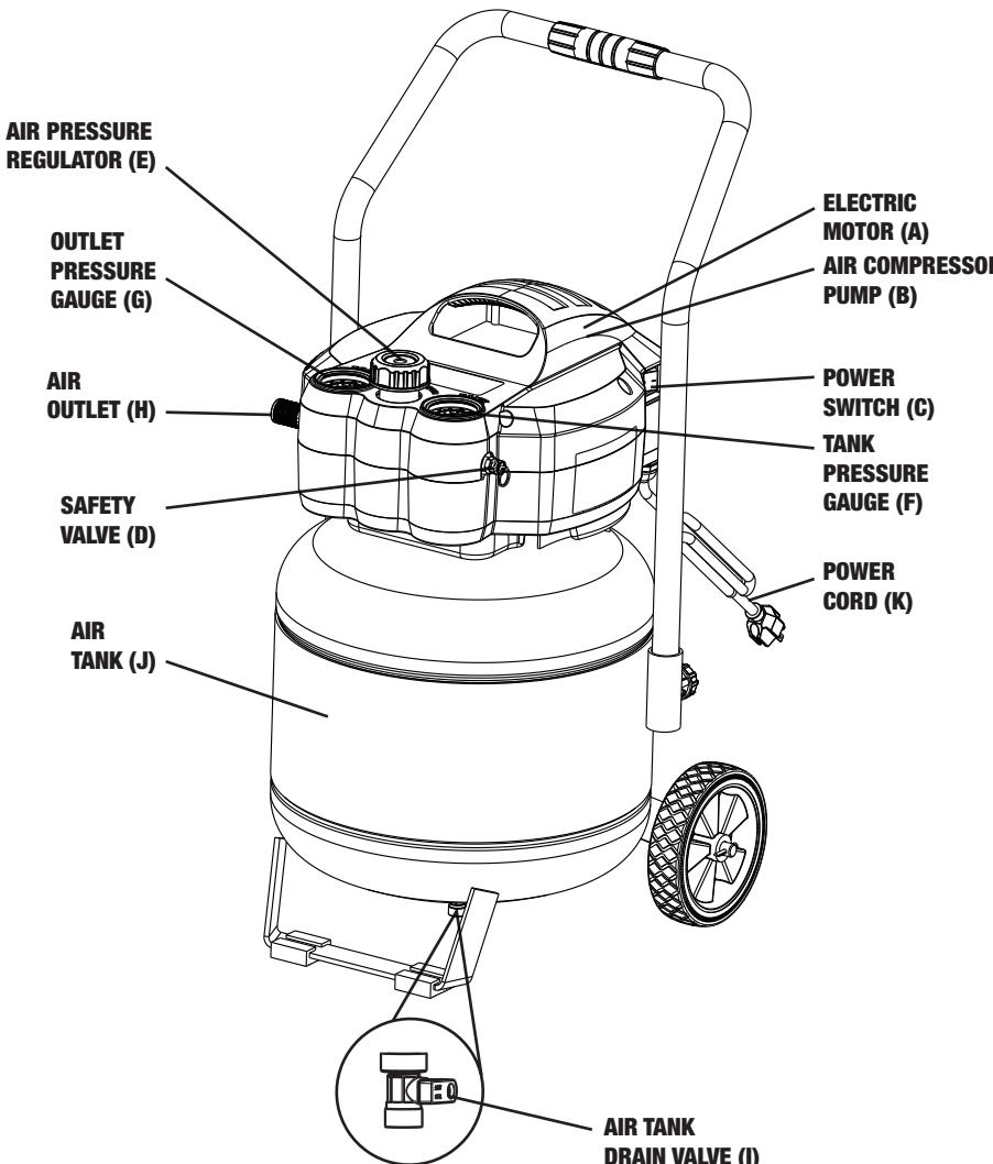
**A. ELECTRIC MOTOR:** The motor is used to power the pump. It is equipped with a thermal overload protector. If the motor overheats for any reason, the thermal overload protector will shut it down in order to prevent the motor from being damaged.
