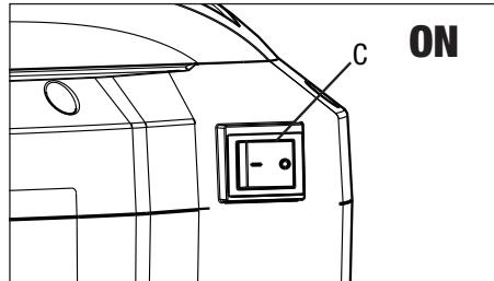
6. After 30 minutes, turn off the pressure switch (C).
