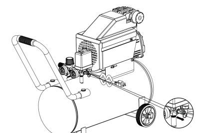
3. Reduce the pressure in the tank through the outlet hose. Pulling the safety valve (D), and keeping it open,
