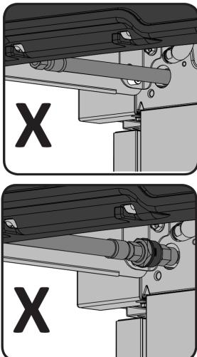
**Fit the orifice into the burner tube and secure with the hose retainer clip supplied. Attach the wire from the manifold to the side burner electrode.**
