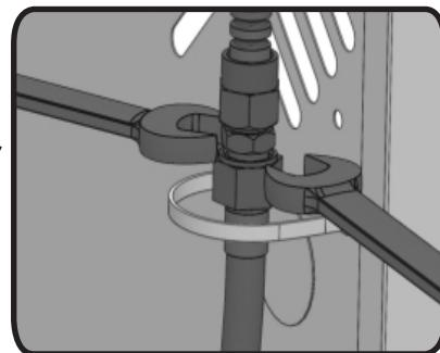
Clip hose to side panel using hose retainer clip supplied.
