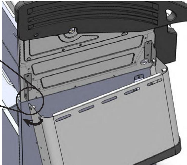
Bend shelf open slightly to insert second pin into bracket.
