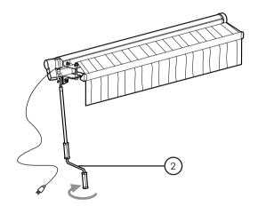
• Turn the crank wand (2) counter-clockwise to retract the fabric.
