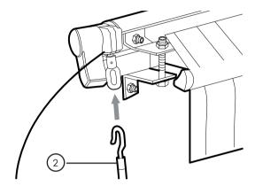
• Turn the crank wand (2) clockwise to extend the fabric.
