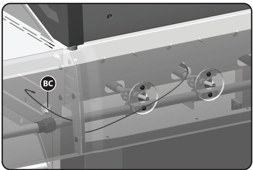
**Attention:** Feed the electrode set (BC) attached to the main burner, through the hole on the left side of the burner box.
