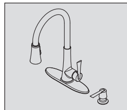
Option 1: 4 Hole With Deckplate Installation
