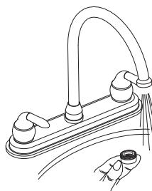
**Important:** After installation is complete, remove the aerator in order to flush the water lines. Turn on the water supply and run for at least one minute. Check for leaks. Re-tighten any connections if necessary. This also flushes away any debris that could cause damage to internal parts. Turn off the water and reinstall the aerator.
