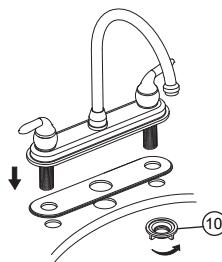
Install new faucet on sink with hot to the left and cold to the right. From under the sink, thread mounting nuts (10) onto faucet. Tighten nuts (10).
