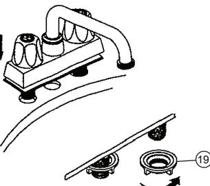
Place new faucet in position on the sink. From under the sink, thread mounting nuts (19) onto faucet. Tighten mounting nuts.
