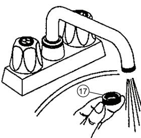
**Important:** After installation is complete, remove the adapter (17) in order to flush the water lines. Turn on the water supply and run for at least one minute. Check for leaks. Re-tighten any connections if necessary. This also flushes away any debris that could cause damage to internal parts. Turn off the water and reinstall the adapter (17).
