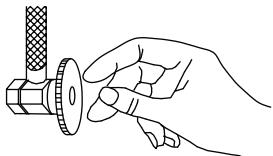
**Shut off water supplies.** Remove old faucet. Clean sink surface in preparation for the new faucet. Make sure to flush the lines properly before installing the new faucet.
