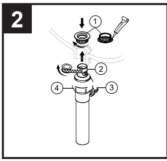
**Installing the pop-up body and pop-up flange**: Apply silicone to the underside of the flange (1). Apply thread sealant tape to the top threads of the body (2) in a clockwise direction. Insert body (2) into sink. Screw flange onto body. Pivot hole (3) must face the back of the sink. Use groove joint pliers to tighten the nut (4), do not overtighten. Do not turn pop-up while tightening nut or sealant may not seal drain.
