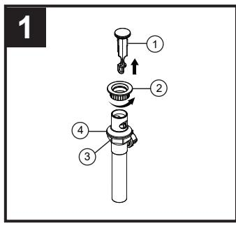
**Preparing for installation of pop-up assembly**: Remove stopper (1) and flange (2). Screw nut (3) all the way down. Push gasket (4) down.
