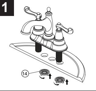
**Shut off water supplies.** Remove old faucet. Clean sink surface in preparation for the new faucet. Flush the lines properly before installing the new faucet. Place the faucet in position on the sink. From under the sink, thread mounting nuts (14) onto faucet. Tighten nuts.
