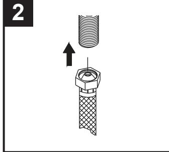
**Stainless Steel Braided Faucet Supply Tubes**: This is the simplest of all installations. If you are using these tubes, this faucet requires one end of the supply tube to have a 1/2" female IPS connection. The other end of this supply tube must match the thread on the water supply fittings or shut off valve under your sink. Once you have identified the required tube, carefully follow the manufacturer's instructions for each tube.
