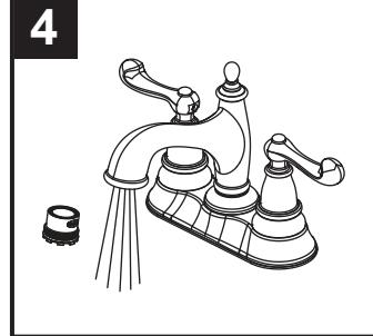
**Important**: After installation is complete, remove the aerator in order to flush the water lines. Turn on the water supply and run for at least one minute. Check for leaks. Re-tighten any connections if necessary. This also flushes away any debris that could cause damage to internal parts. Turn off the water and reinstall the aerator.
