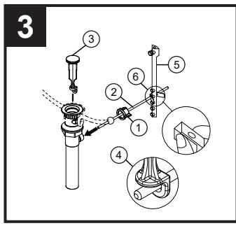
**Installing the horizontal rod, stopper and strap**: Remove pivot nut (1). Install horizontal rod (2) and stopper (3) as shown (4). Hand tighten pivot nut (1). Attached horizontal rod to strap (5) using clip (6).
