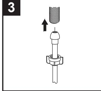
**Ball Nose Flexible Supplies**: If you are using these supplies to connect the faucet to the water lines; slip coupling nut behind ball-nose of flexible supply tube. Ball nose coupling will go partially into 1PS shank or fitting. Tighten coupling nut (do not overtighten). Install opposite end according to manufacturer's instructions for both tubes.
