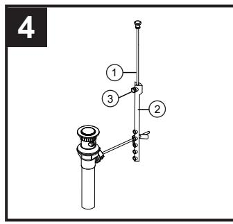
**Installing the lift rod**: Insert lift rod (1) through faucet and into strap (2). Tighten screw (3). **Adjusting the lift rod**: Adjust lift rod function by adjusting location of thumb screw along the lift rod or by adjusting the hole in which the ball rod goes through the strap. Be sure to leave enough space between lift rod know and faucet spout when rod is down.
