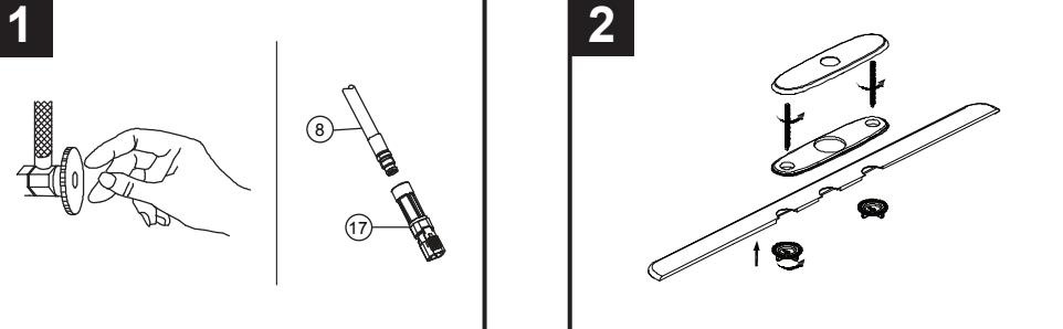
**Shut off water supplies.** Remove old faucet. Clean sink surface in preparation for the new faucet. Flush the lines properly before installing the new faucet. Before installation, remove quick connector (17) from the free end of the pull-out hose (8).
