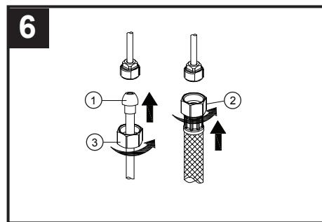
Make connections to water lines. Use 1/2" I.P.S. faucet connections (2) or supply line coupling nuts (3) (not included) with a 3/8" O.D. ball-nose riser (1). Use wrenches to tighten connections. Do not overtighten.
