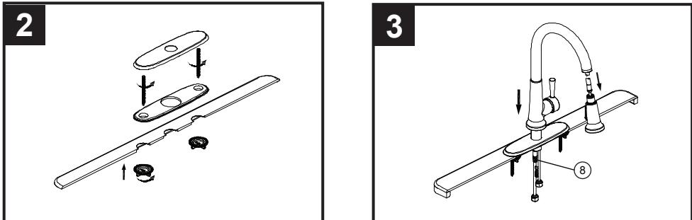
Retract pull-out hose (8) up through faucet body until the pull-out hose fitting is flush with the bottom of the shank. Do not pull hose fitting past the shank. Insert faucet body through the hole in the escutcheon. **Note:** Do not feed the pull-out hose (8) back down through the spout until step 5.
