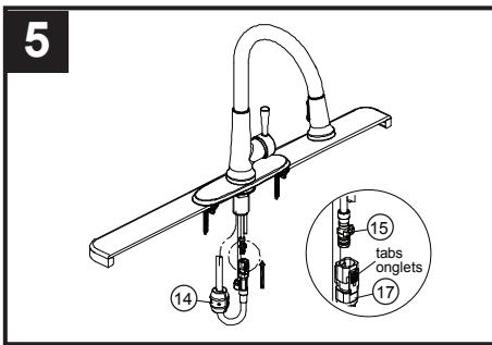
Push the quick connector (17) firmly upward and attach it to the receiving block (15). Pull down moderately to ensure the connection has been made. If it is necessary to remove the quick connector (17), squeeze the tabs on the hose and then pull down to disconnect. After connecting the hose, attach weight (14) at the bottom of the hose loop to prevent hose from twisting and return it to the proper position.
