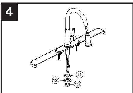
Install the rubber washer (11) and metal washer (12) onto the threaded mounting shank. Thread the nut (13) onto the mounting shank. Do not overtighten.
