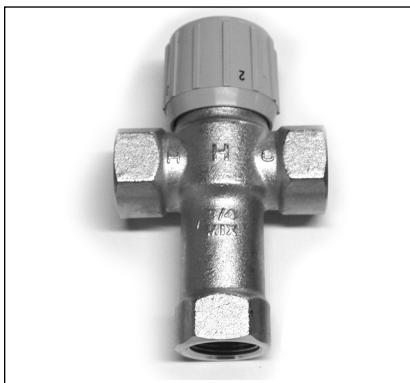
Figure 7 - Thermostatic Mixing Valves installed at each point-of-use can help prevent scalding. Install Thermostatic Mixing Valves (figure 7) to regulate the temperature of the water supplied to each point-of-use (for example, kitchen sink, bathroom sink, bath, shower). Consult the valve manufacturer's instructions or a qualified person.
