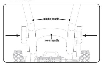
Attach the left handle and right handle to the middle handle using the knobs and bolts provided.
