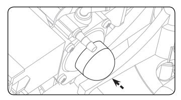
6. Press and hold the fuel button while you press the primer bulb one to two times again.
