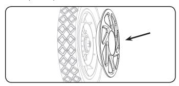
6. Attach wheel assembly to main body, reverse steps 1-2.
