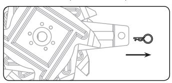
2. Remove the clevis pin from the axle assembly.
