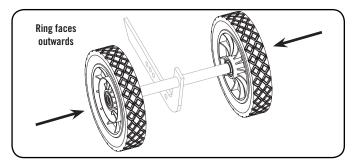
4. Slide a washer onto the axle on each side. Add the nut and hand tighten.
