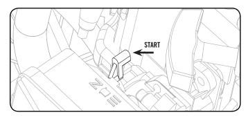
5. Locate the primer bulb on the upper right of the engine, in front of the fuel tank. Press the primer bulb until you see fuel flow through the clear fuel return line. Starting the engine "cold," press the primer bulb five times.
