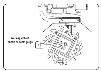
Remember, any cultivator will tangle in tall grass, stringy vines, or overly large weeds. So, if you plan to cultivate in these conditions first use a pruner or brush cutter to chop up the overgrowth. If the tines become tangled, turn the engine off and allow the tines to full come to a stop before trying to clear them.
