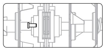
3. Place wheel on each end of the axle. Note installation direction - ring faces outwards.
