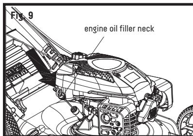
1. Remove the oil filler dipstick and wipe oil from it with a clean cloth (see Fig. 9).
