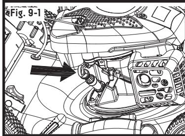
3. Remove the dipstick and check the oil level: the oil level must be between the Min and Max marks on the dipstick. If near the lower level, fill to upper level with the recommended oil (SAE30 or equivalent). Do not overfill. Wipe away any spilled oil (see Fig. 10).
