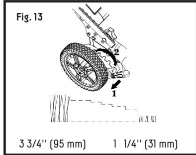
The cutting height is centrally adjusted with cutting height adjusting handle. Different cutting heights can be selected.
