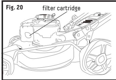
1. Use a screwdriver (not provided) to loosen the screw then remove the cover.
