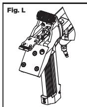
3. Pull out and lift up the cover plate. Remove it to clean the jam (Fig. K&L).
