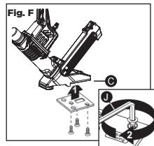
6. Using the hex key (J), hold the nailer upside down and remove the three screws from the base plate by turning counter clockwise. Attach the desired plate (See Fig. F). Ensure the screw holes on the base plate line up with the holes at the nailer base (C). Tighten the screws by turning clockwise (See Fig. F). Make sure screws do not protrude out of the base plate.
