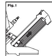
**NOTE:** Test the driving depth using a scrap piece of wood before working on the workpiece. If the fasteners are being driven too deep or not deeply enough, adjust the spacer wheel in order to provide more or less air pressure, as required.
