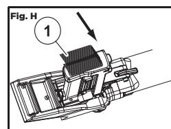
2. Staples: Insert the staples (1) from the top area of the magazine with one arm of the staple in the center slot of the magazine and the other arm along the left side of the magazine (Fig. H).
