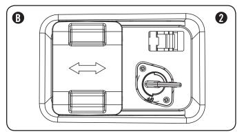
To turn a fuel valve to the off position the valve must be in the horizontal position. (2)
