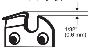
Raker (depth gauge) clearance
