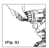
**NOTE:** This device is fitted with a spindle lock and rotating the chuck is a one-handed operation.
