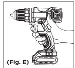
**NOTE:** The drill will not run unless the direction of forward/reverse selector is engaged fully to the left or right.
