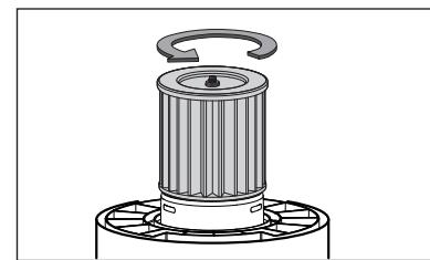
5 Slide cartridge filter off filter cage.
