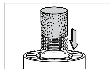
7 For wet vacuum cleaning, install the supplied foam filter.
