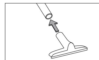
10 Fit the required accessory on to the suction tube.
