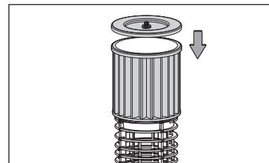
2 Place retainer on top of cartridge filter against hole of basket.
