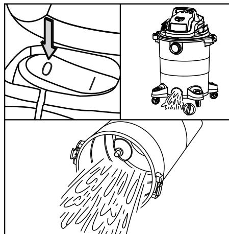
**6** After use, flip the switch to the "O" position and unplug the power cord, then empty and dry the tank.
