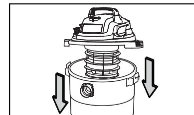
2 Ensure that the cartridge filter is completely mounted.
