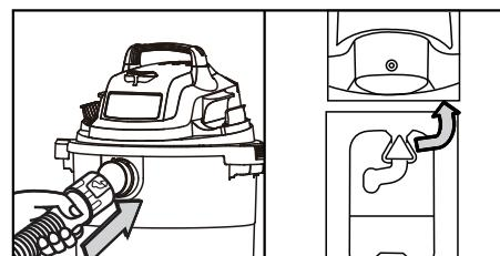
9 Insert the large end of the hose into the front inlet of the tank and turn to lock.
