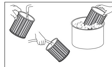
7 When wet (to prevent mould and/or mildew build-up), the cartridge filter should be moved and allowed to air dry for a 24-hour period before being re-installed back onto the filter cage.
