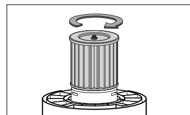
3 To secure filter; put on retainer nut and turn clockwise to tighten until snug. Do not over tighten.
