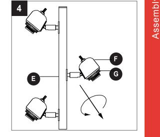
5. Attach plastic shades (H) to sockets (F). Secure with socket rings (G).
