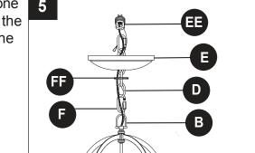
3. Weave electrical wires and ground wire up chain (D), through nut (FF), through screw collar loop (EE), through threaded tube (BB), through canopy (E) and
