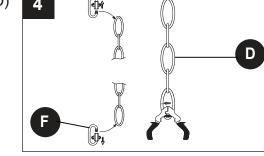
5. Attach one K/D ring (F) to the loop (B). Place the other one through the nut (FF) and canopy (E), then attach it to the screw collar loop (EE). Screw the K/D rings (F) until the chain (D) is firmly secured.
