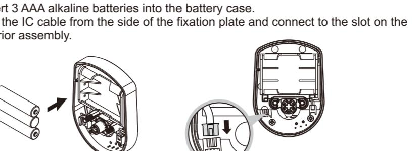
Insert 3 AAA alkaline batteries into the battery case. Pull the IC cable from the side of the fixation plate and connect to the slot on the interior assembly.
