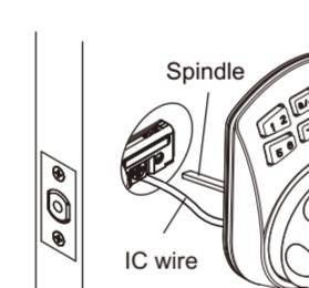
Left handed door install the spindle (vertically)
