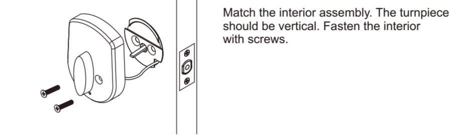
Match the interior assembly. The turnpiece should be vertical. Fasten the interior with screws.
