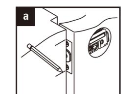
To identify the centre of strike: close the door so the latchbolt is against the door frame. Mark the centre line on the doorframe exactly opposite the latch hole in the door edge.
