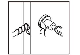
Using the marks as a guide to drill a hole Ø2 1/8" (54 mm) through the door face for the lockset, then a hole of Ø1" (25.4 mm) for latch.
