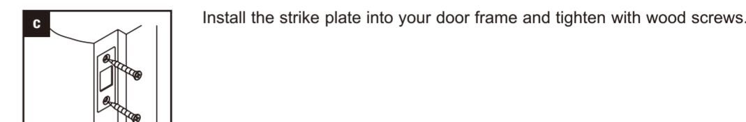
Install the strike plate into your door frame and tighten with wood screws.
