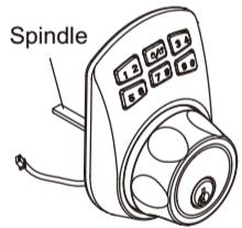
Left handed door install the spindle (vertically)
