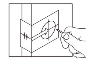
Select the height and backset as desired on the door face; use the TEMPLATE as a guide to mark the centre of the circle on the door face and the centre of the door edge.
