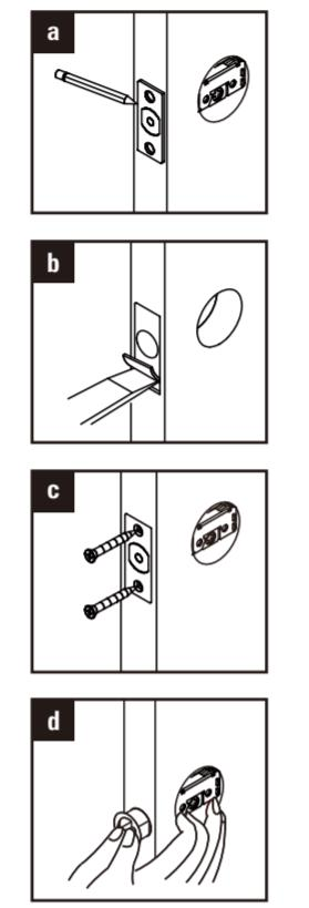
Insert the latch and ensure it is parallel to the door face. Mark the outline of the faceplate, then take out the latch.
