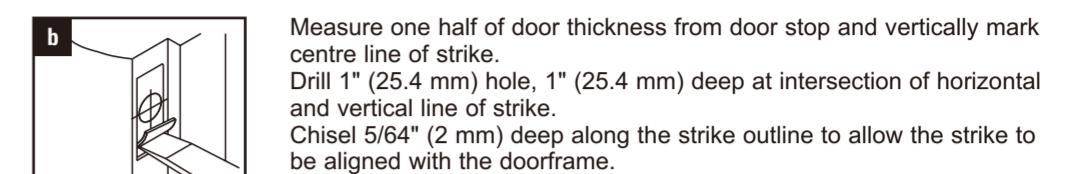
Measure one half of door thickness from door stop and vertically mark centre line of strike. Drill 1" (25.4 mm) hole, 1" (25.4 mm) deep at intersection of horizontal and vertical line of strike. Chisel 5/64" (2 mm) deep along the strike outline to allow the strike to be aligned with the doorframe.
