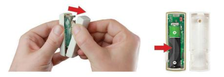
2. Use a coin to open the Motion Sensor and insert an AA-Battery.
