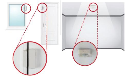
The motion sensor can be mounted with a double-sided tape or screws on a ceiling. It can be also installed to monitor or protect
