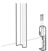
Run the wires up the wall and T-rail to the garage door
