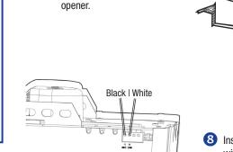
8 Insert the wires by colours: white with white, black with black all the way into "safety beam" ) ( terminals.
