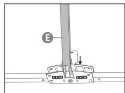
Insert the one top and two bottom quick release pins (1) into the corresponding keyholes on the centre bracket.
