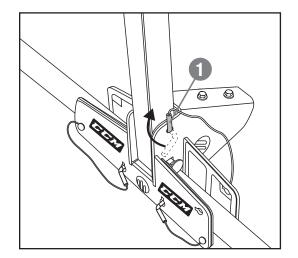
Hold the centre mast (E) and remove the top quick-release pin (1) from the bike carrier.
