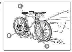
Push down the rack arm (9) of the centre mast onto the top tube (10) of the bicycle until the rack arm gets locked in its position.
