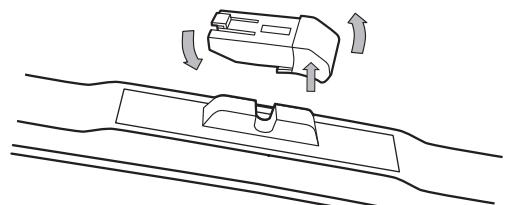
For arm types above, remove the adapter and reattach in the opposite direction.
