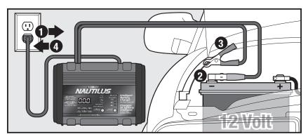
**1 Before** connecting and disconnecting the DC output clamps, remove the AC plug from the electrical outlet.
