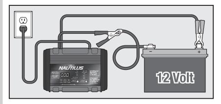
IMPORTANT NOTE: If your charger detects ANY problems with the battery you are attempting to charge, it WILL show a fault code in the Digital Display and WILL NOT begin charging automatically.
