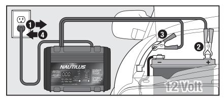
**Before** connecting and disconnecting the DC output clamps, remove the AC plug from the electrical outlet.
