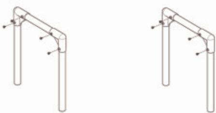
**4. Attach the side frames to rest of the unit:**
