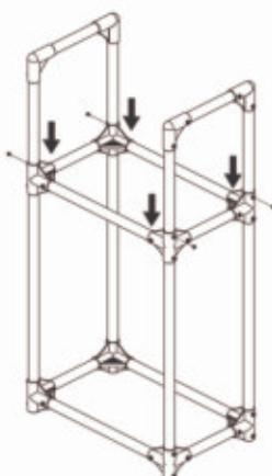
**5. Insert and tighten all screws.**
