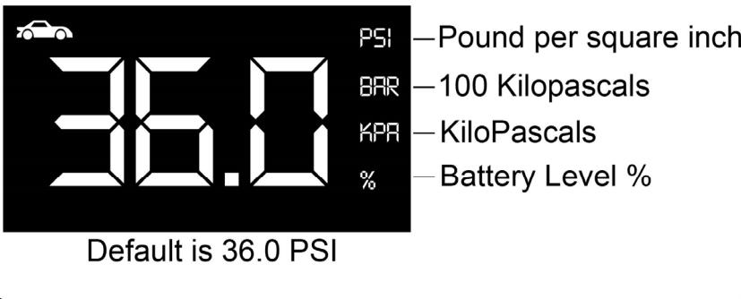
5) The default setting is 36.0 PSI. To change from PSI/BAR/KPA simply press the “**Inflator mode**”
