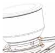
Fig. 2: Align the positions in red circles in the Figure, and press it down, rotate it clockwise and install it into the machine.
