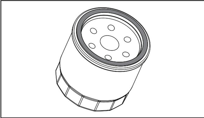
6. Install new oil filter by turning clockwise by hand until gasket contacts the engine block. Then apply additional 3/4 turn.
