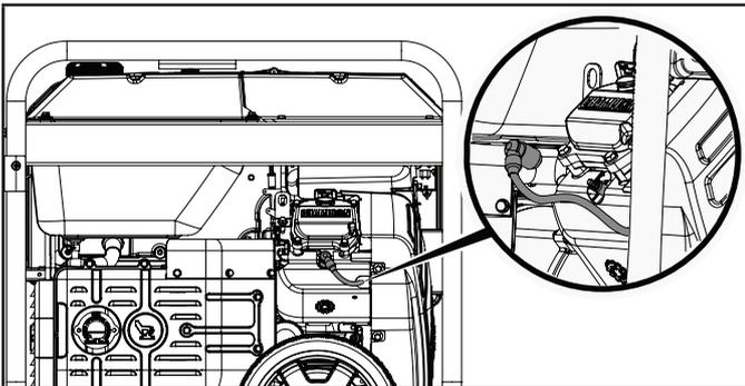
2. Use a spark plug socket tool (not included), or a 13/16 in. (21 mm) socket (not included) to remove the plug.
