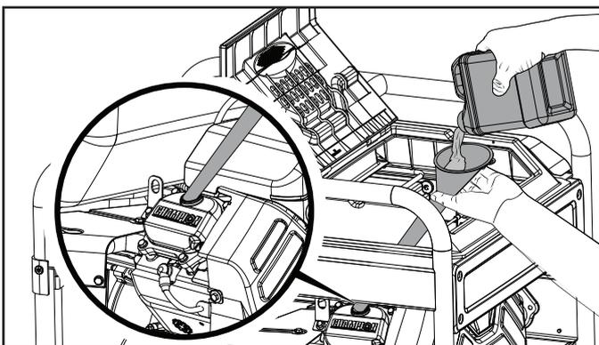
5. Pull out dipstick and check engine oil level. Add as needed. **DO NOT OVERFILL.**
