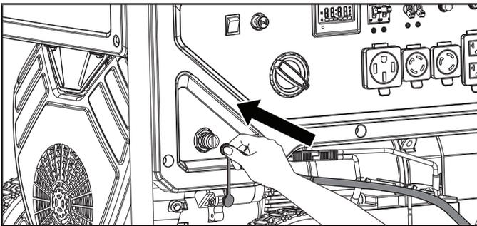
5. Before operation, open the NG supply line and check for leaks. Use a soapy water mixture to verify all connections prior to starting the generator. If soapy bubbles are present indicating leaks turn off the NG supply and do not start generator. Recheck connections and tightness and turn NG supply valve back on and repeat soapy water mixture on connection fitting. If the NG leak continues do not use the generator and contact a qualified technician for repair.
