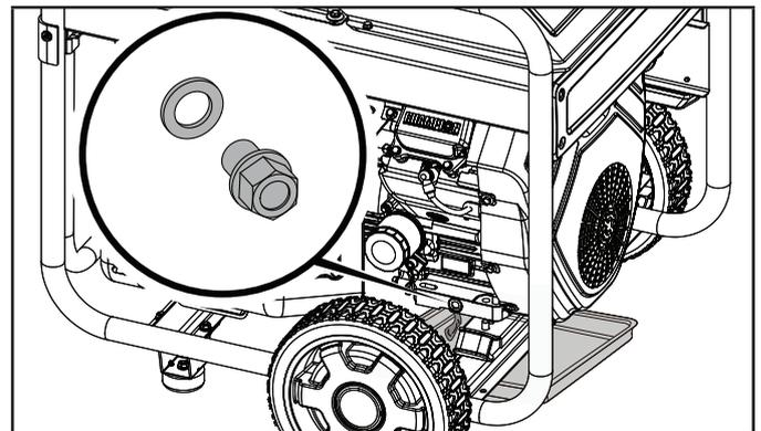
3. Replace the oil drain bolt.
