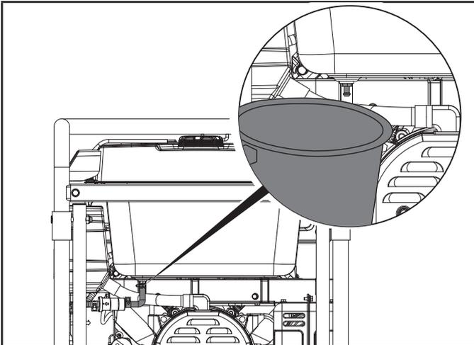
3. When gasoline stops flowing from the fuel tank, return fuel hose and clip to fuel tank fitting. Properly dispose of the drained gasoline according to local regulations or guidelines.
