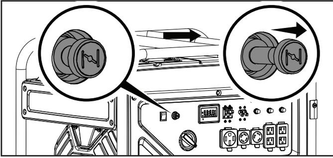
5. Press and hold the ignition switch to the "START" position. Release as the engine begins to start. If the engine fails to start within five seconds, release the switch and wait at least ten seconds before attempting to start the engine again.
