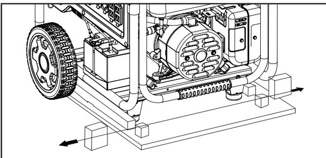
9. Raise handle and pull generator forward until wheels touch the ground. Then pull generator out from wood pallet.
