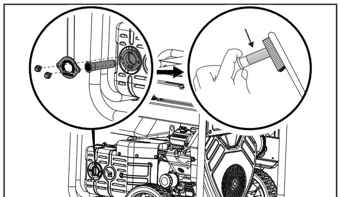
5. Replace the spark arrestor if it is damaged.
