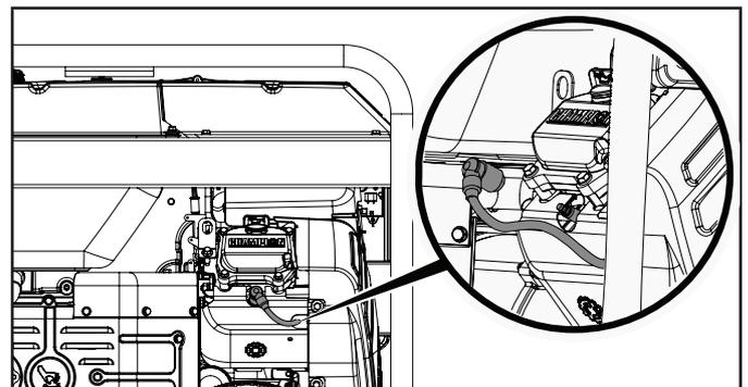
10. Install the spark plug on each cylinder but DO NOT install spark plug cap.
