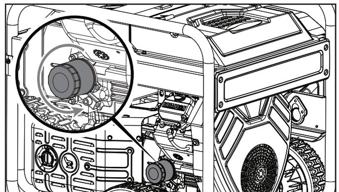
5. Apply a light coat of clean oil onto the gasket of new oil filter.
