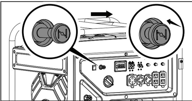
9. Press and hold the ignition switch in the “START” position for up to 5 seconds or until started.
