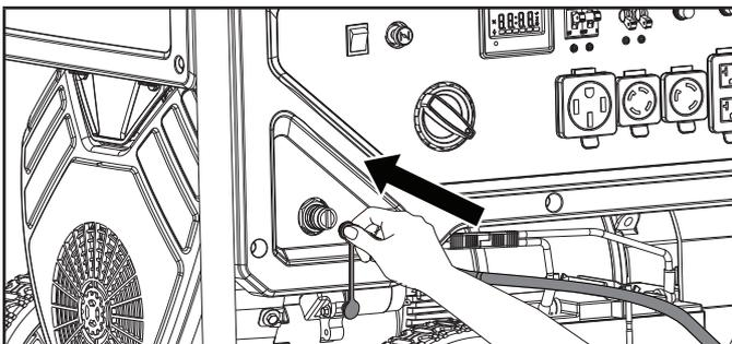
4. Connect the other end of the LPG hose to the LPG cylinder valve and hand tighten.
