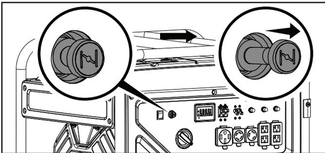
7. Press the ignition switch to the "START" position for 2-3 seconds.
