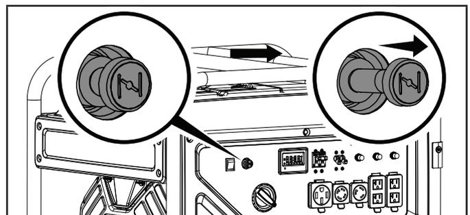
7. Press the ignition switch to the “START” position for 2-3 seconds.
