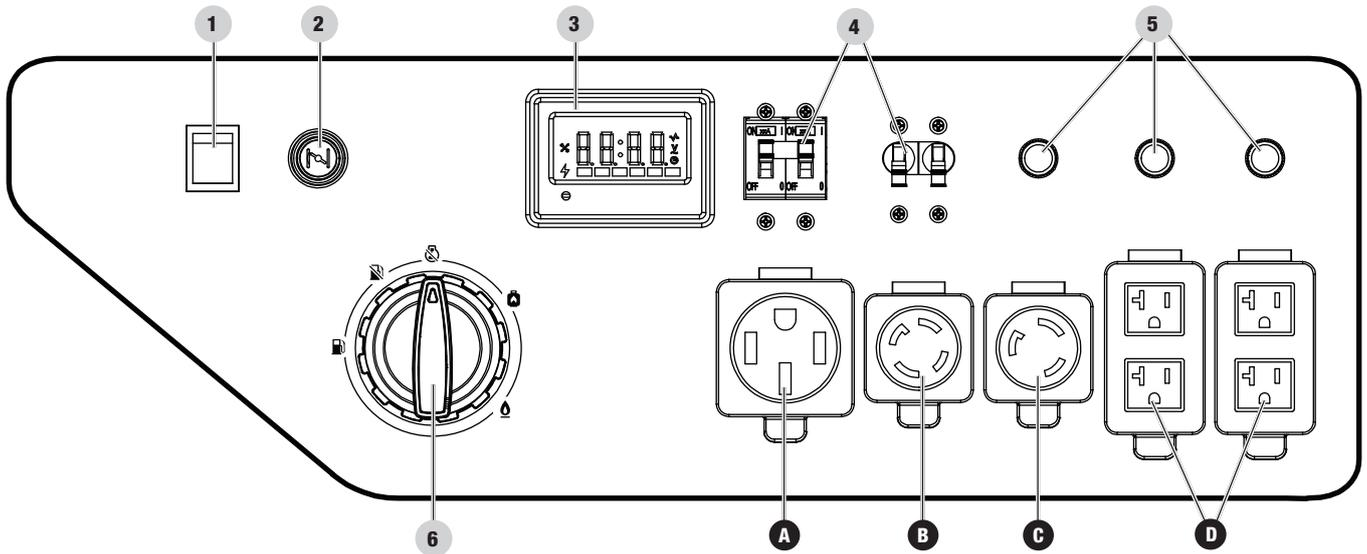
1. **Ignition Switch** – Used for electric starting of the generator.
