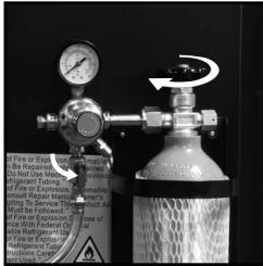
Close the Shut Off Valve on the Regulator, and open the CO<sub>2</sub> Tank valve completely by turning it counter-clockwise.
