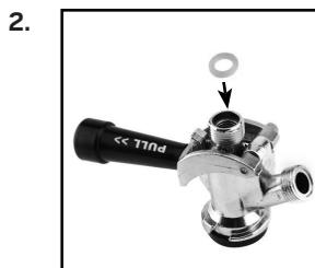
Remove the black packing cap from the top of the Coupler, then place the Top Coupler Washer flush and centered on the top of the Keg Coupler.
