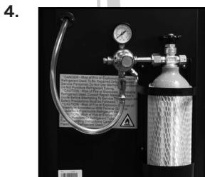
Place the CO<sub>2</sub> Tank into the CO<sub>2</sub> Tank Holder.
