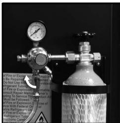
Once desired pressure is reached, tighten the inner Locking Ring. Pull the PRV to assure the correct setting. If necessary, readjust your settings.
