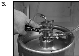
Make sure the Tap Tower is in the closed (handle pointing straight up) position. Secure the connection by pulling the Coupler handle out and pushing down until it locks into position. The pull handle will "click" when it shifts into the final downward position. This will open the beer and CO<sub>2</sub> gas valves. The Keg is now tapped.
