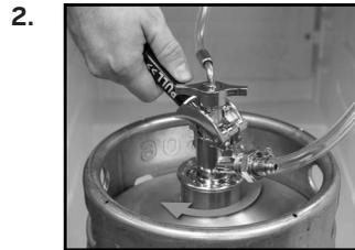
Turn the Coupler clockwise until it locks securely into position.
