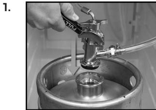
Make sure the black pull handle of the Coupler is in the open (up) position, then insert the Coupler into the locking neck of the beer keg.
