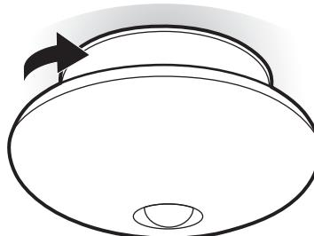
Motion Sensor will turn fixture on when motion is detected up to 9 feet away from fixture. Fixture will turn off after 10 minutes if no motion is detected. Sensitivity of motion sensor will be affected by obstructions such as walls, doors, etc. Relocate the fixture to a different socket if obstruction prohibits operation of the sensor.
