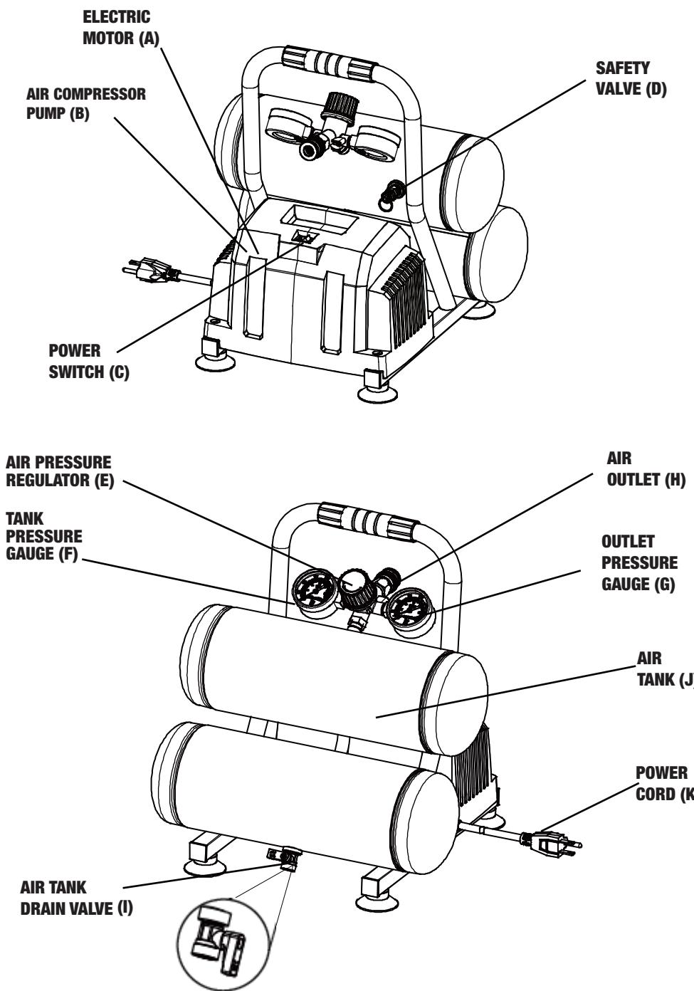
**A. ELECTRIC MOTOR:** The motor is used to power the pump. It is equipped with a thermal overload protector. If the motor overheats for any reason, the thermal overload protector will shut it down in order to prevent the motor from being damaged.
