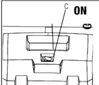
6. After 30 minutes, turn off the power switch (C).
