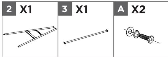
Attach the support frame **3** to the table leg **2** using the screws **A** with spring washers and washers, aligning the holes.
