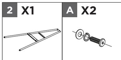
Connect the table leg **2** to the assembled frame using the screws **A** with spring washers and washers, aligning the holes.
