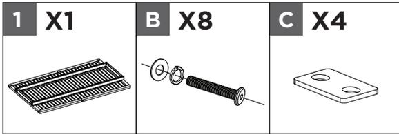
Connect the table top **1** to the assembled frame using the support plate **C** and the screws **B** with spring washers and washers, aligning the holes.
