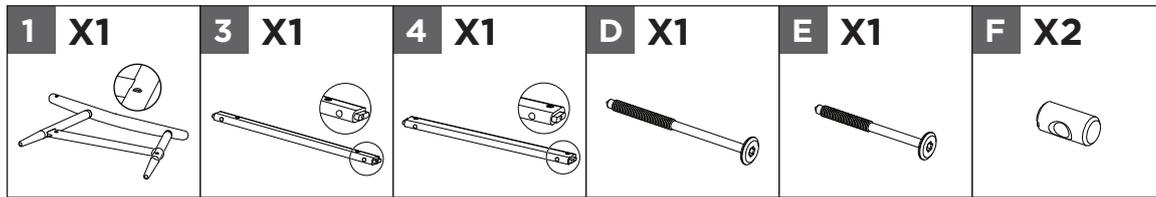
Attach the right arm **1** to the bottom panel **3** and **4** using the barrel nut **F** and screws **D** and **E**, aligning the holes.
