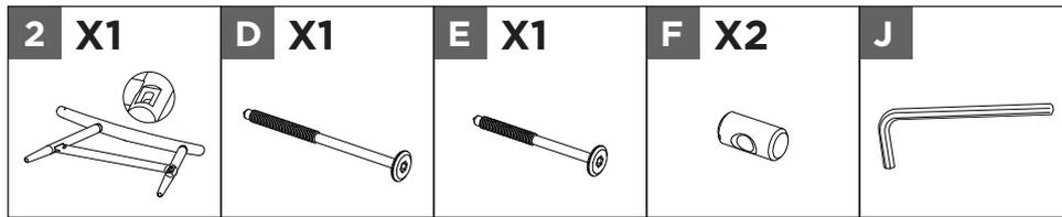
Connect the left arm **2** to the assembled frame using the barrel nut **F** and screws **D** and **E**, aligning the holes.
