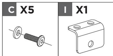
Connect using the screws **C** with washers and the L bracket **I**, aligning the holes.
