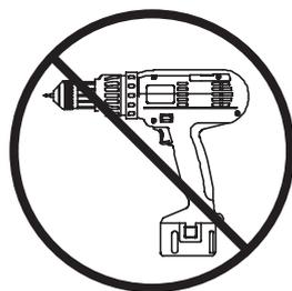
**NOTE:** A drill is not recommended; be aware of over-drilling in order to avoid damage
