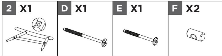
Connect the left arm **2** to the assembled frame using the barrel nut **F** and screws **D** and **E**, aligning the holes.
