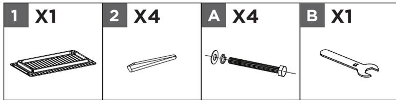
Attach the table leg **2** to the table top **1** using the screws **A** with spring washers and washers, aligning the holes.
