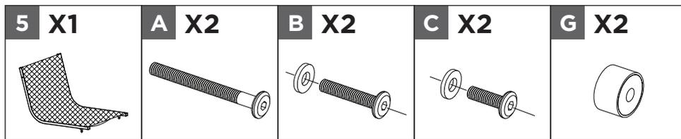
Connect the seat panel **5** to the assembled frame using the screws **B** with washers and the spacers **G**, and then using the screws **C** with washers, finally using the screws **A**, aligning the holes.
