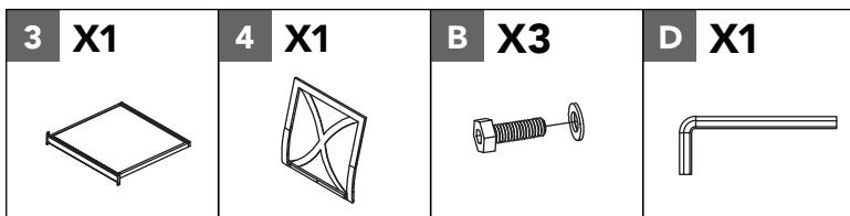
Attach chair back (4) to the chair seat (3) using the M6x25L combination bolts with washers (B), aligning the holes. Do not tighten completely.
