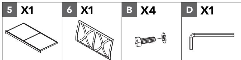
Attach loveseat back (6) to the loveseat seat (5) using the M6x25L combination bolts with washers (B), aligning the holes. Do not tighten completely.
