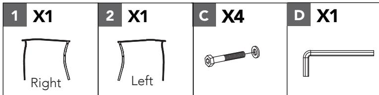
Line up the bolt holes on the right arm (1) with the corresponding bolt holes on the back frame (6) and insert the M6x55L combination bolts with washers (C).
