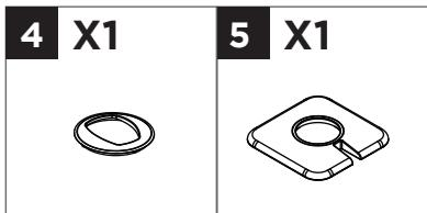
Slide the lower base cover **5** and the upper base cover **4** onto the base tube **3**.
