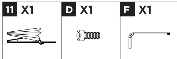
Connect the umbrella shade **11** to the base tube **3** using M6x15 bolts **D** with M6 hex key **F**.
