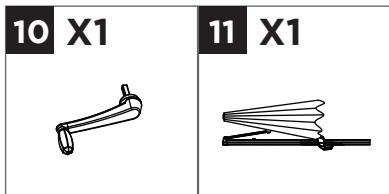
Slowly turn the crank **10** in a counter-clockwise direction to close the umbrella. Press the button on the umbrella shade **11** and push down.
