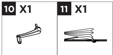
Press the button on the umbrella shade **11** handle and push up to the desired position. Attach the crank **10** to the umbrella shade **11**.
