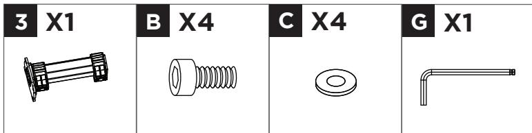
Attach the base tube **3** to the turn plate **7** by using M10x20 bolts **B**, flat washers **C** with the M10 hex key **G**.
