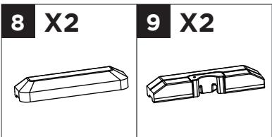
Open the side bases **8** and the middle bases **9** by twisting the plugs in a counter-clockwise Pour sand or limestone into the side bases **8** and the middle bases **9**. Close the side bases **8** and the middle bases **9** by twisting the plugs in a clockwise direction.
