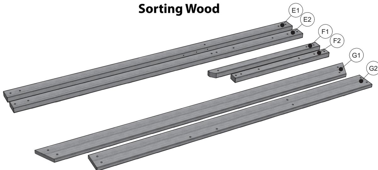
When removing the wood from the boxes we recommend arranging them by part number before you begin assembly. This will allow for faster assembly and easily identify any parts that may be missing or damaged.
