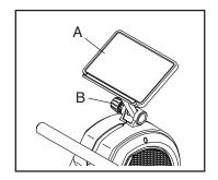
To adjust the angle of the tablet holder (A), first hold the tablet holder with one hand, and loosen the adjustment knob (B) with your other hand. Raise or lower the tablet holder, and then firmly tighten the adjustment knob.
