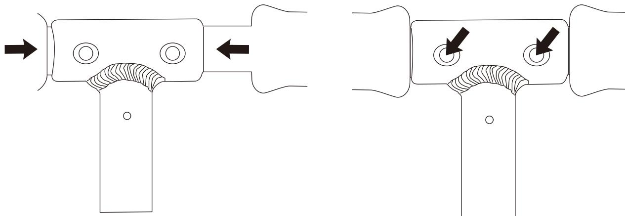
Please ensure the handlebar pins are locked, riding with thumbs on the pins can cause the handlebars to come off.
