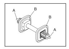
each side of the dumbbell; make sure to place the same number of weight plates on both sides of the dumbbell. Then, turn the knobs to the locked position; make sure that the knobs are securely in the locked position before you use the dumbbell.
