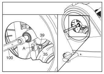
Plug in the power adapter and rotate the Left Crank Arm (100) for a moment. Repeat these actions until the console displays correct feedback.
