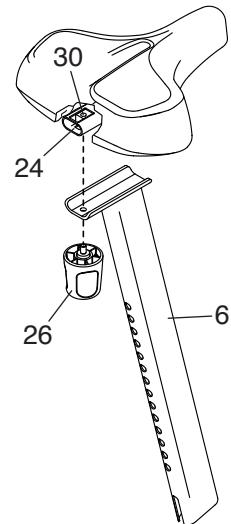
10. Loosen the Seat Post Knob (27) and pull it outward. Next, insert the Seat Post (6) into the Seat Post Sleeve (28), and then release the Seat Post Knob. **Move the Seat Post upward or downward slightly to make sure that the Seat Post Knob is engaged in one of the adjustment holes in the Seat Post. Then, tighten the Seat Post Knob.**
