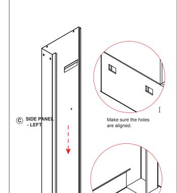
Make sure that the side panel is inserted into the gaps
