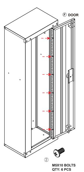
Install the Door onto the cabinet using M5X10 bolts.Make sure there is about 2 mm (1/16") space between the Door and the cabinet.
