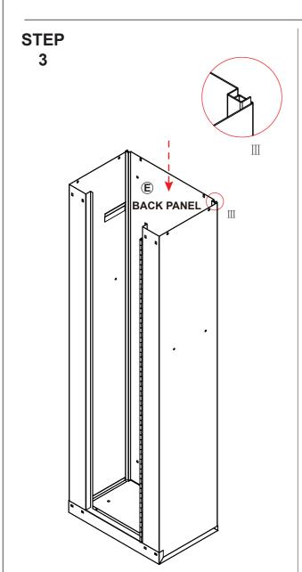
As shown, insert the Back Panel between the two sides until the top is aligned.
