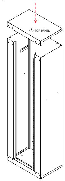
Install the Top Panel onto the Side Panels and Back Panel. Please refer to the Bottom Panel for the position. A rubber mallet can be used to align the top flush with the Side and Back Panels.
