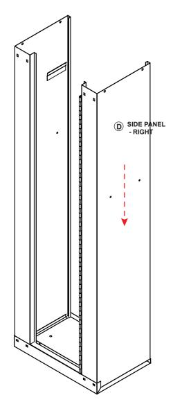
Assemble Side Panel-Right with Bottom Panel, Same as STEP 1, Set the Side Panel-Right down into the Bottom Panel.
