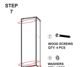
Use the wood screws and washers to secure the cabinet to floor or wall.
