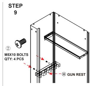
Install the gun rests with M5X10 bolts on both Side Panels.
