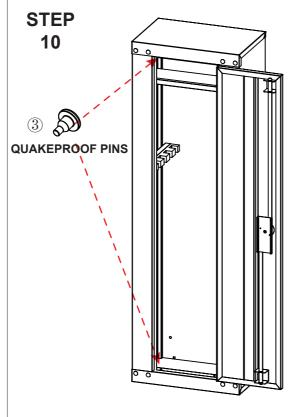
Install the Quakeproof Pins through the pre-drilled holes, and check that all the nuts have been tightened.
