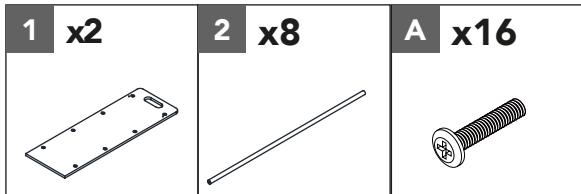
Attach eight metal tubes (2) to side panels (1) using sixteen bolts (A).
