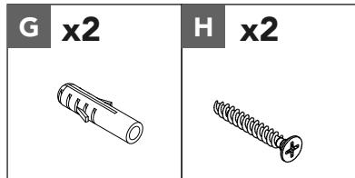
Attach the product to wall using two wall plugs (G) and two screws (H).
