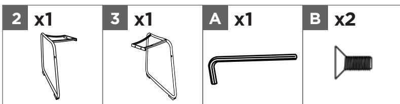
Attach left leg 3 to right leg 2 with the bolts B as shown. The bolts must go through holes on left leg 3 first and then screw into the threads on right leg 2.
