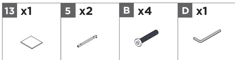
Insert four bolts M6x30 **B** through two support bars **5** into shelf **13**. Tighten all bolts with hex key **D**.
