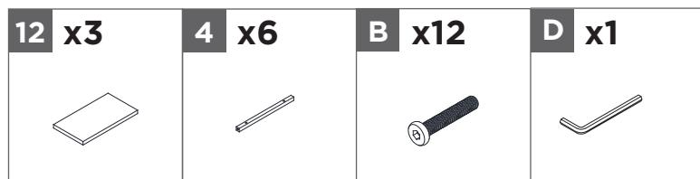
Insert four bolts M6x30 **B** through two support bars **4** into shelf **12**.
