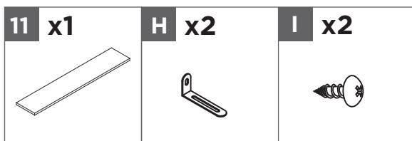
Insert two screws **I** through anti-tip brackets **H** into top panel **11**. Tighten all screws.
