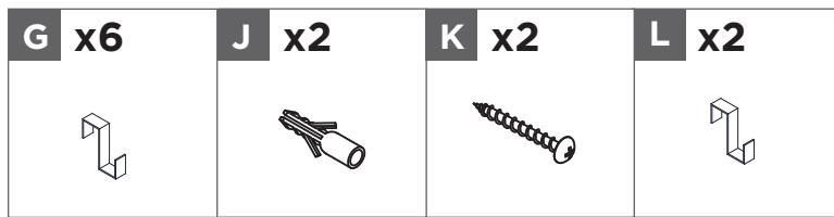
Using the anti-tip brackets as a guide, mark two spots on the wall. Drill a hole at each mark on the wall stud, hammer two wall anchors **J** into the wall, and fasten the anti-tip brackets using two screws M4x35 **K** screwed into the wall anchors **J**. Tighten all screws.
