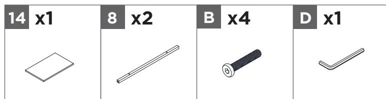
Insert four bolts M6x30 **B** through two seat plate support bars **8** into seat plate **14**. Tighten all bolts with hex key **D**.
