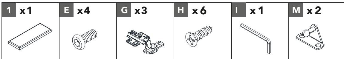
Align 3 hinges **G** with the holes on the seat panel **1**. Attach with 6 screws **H**.
