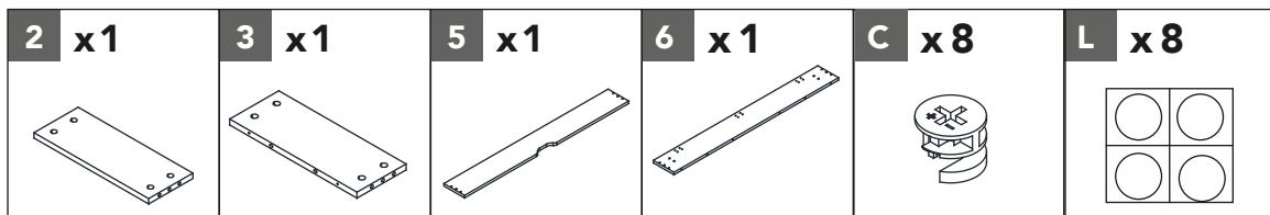
Connect front panel **5** and back panel **6** with left side panel **2** and right side panel **3** using 8 cam locks **C**. Cover the cam lock holes in the side panels with coated paper stickers **L**.
