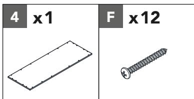
Attach the bottom panel **4** to the assembled wood frame using 12 screws **F**.
