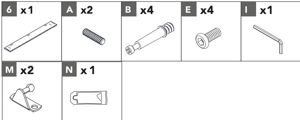
Insert 2 wood dowels **A** and 4 cam bolts **B** into back panel **6**. Attach 2 gas spring connectors **M** into the back panel **6** using 4 bolts **E**.
