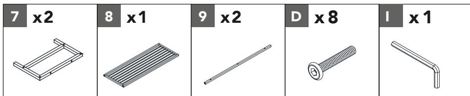
Align the metal shelf **8** and two metal support rails **9** with the holes on the two metal legs **7**. Attach them with 8 bolts **D**. Use hex key **I** to tighten the bolts.
