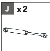
Attach 2 gas spring lid stays **J** into the gas spring connectors **M**.
