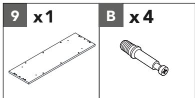
Insert four cam bolts (B) into the fixed shelf (9).
