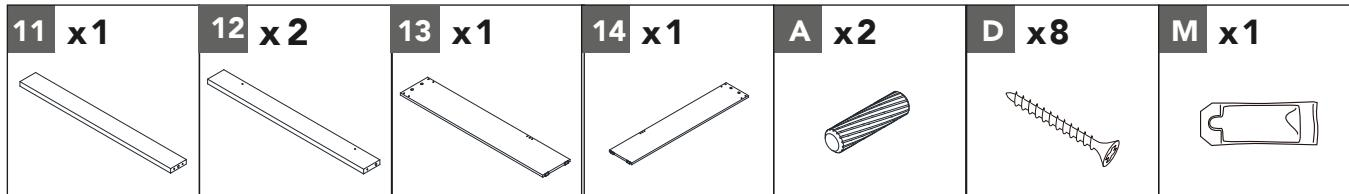
Align the dowels on the strip (11) and trim (12) with the holes on the lower left side panel (13) and lower right side panel (14). Attach them with eight screws (D).
