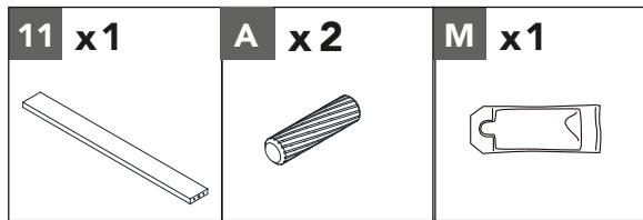
Insert two wood dowels (A) onto the ends of the strip (11).
