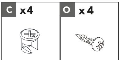
Insert four cams (C) into the holes of lower left side panel (13) and lower right side panel (14). Align the cam bolts (B) on the fixed shelf (9) with the holes on the lower left side panel (13) and lower right side panel (14). Twist the cams (C) to secure.
