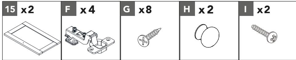
Align two hinges (F) with the holes on the door panel (15). Attach them with four screws (G). Align 1 door knob (H) with the holes on the door panel (15). Attach with 1 screw (I). Repeat this step once more to prepare the second door.
