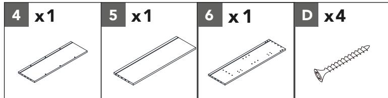
Align the dowels on the fixed shelf (5) and top (4) with the holes on the upper right side panel (6). Attach them with four screws (D).
