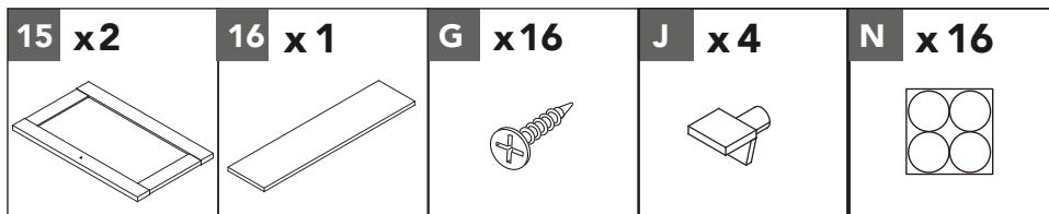
Attached two door panels (15) into the upper right side panel (6) and upper left side panel (7) with 16 screws (G).
