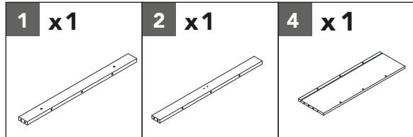
Align back trim (1) and front trim (2) with the holes on the top (4). Connect them with wood dowels.
